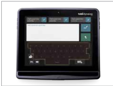
The "dwell-free typing" keyboard gives literate users the chance to increase their typing speed by 50-100 percent.*
